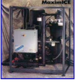
Thermal energy storage systems can reduce the refrigeration equipment used in conventional cooling systems and offer lower running costs. The pumpable characteristics of Slurry-ICE offer reduced pumping energy, smaller pipe sizes and the most economical capacity and duty balancing for any given application.
