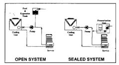
Figure 2: Circulation system types
